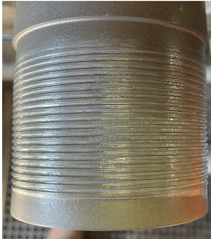
Figure 3: Example of Proper & Acceptable Thread Compound Application of the Pin Connection
