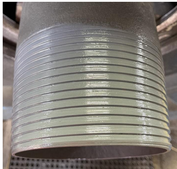
Figure 3: Example of Proper Thread Compound Application of the Pin Connection
