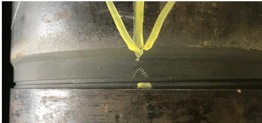
Figure 9: Example of Proper Triangle Stamp Position After Make-Up
