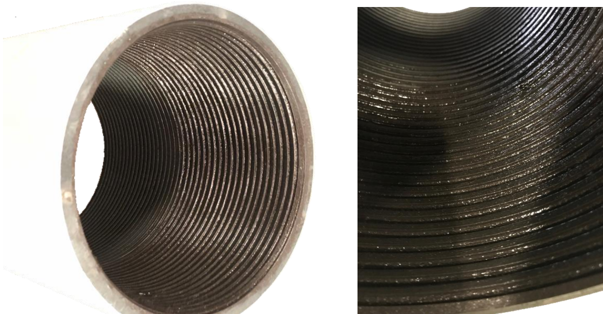
Image 1: Correct way to apply thread compound
